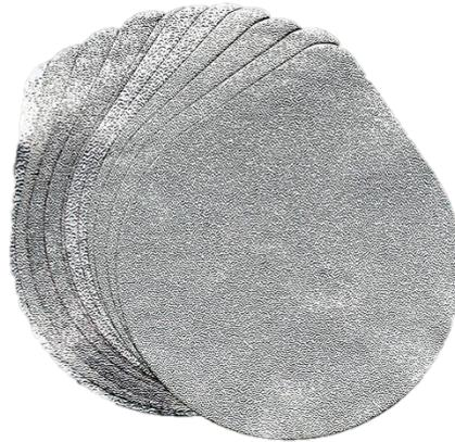
The foils are printed on one side and with a sealant polymer film or heat seal lacquer on the other side for seal ability with the substrate. It enables the user to open the pack with minimal force and also prevent spillage. The foil comes available with barrier variants to prevent contamination of the contents in the container. The foils are suitable for sealing containers made from PS / PVC / PET and PP.
